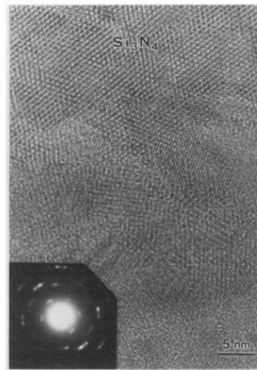
Fig. 5. HRTEM photograph of the transition region from silicon nitride to the amorphous layer. The nanocrystalline layer is observed in between them. The diffraction pattern is from the nanocrystalline layer. The incident electron beam is along the \langle 001 \rangle axis of silicon nitride.
